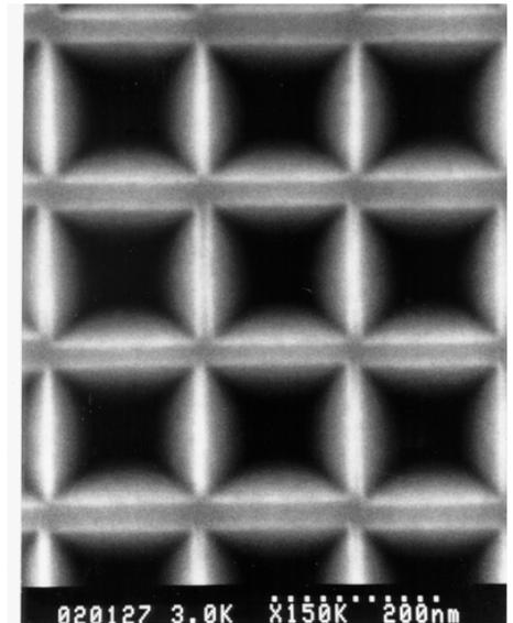
(200-nm size pyramidal pit on (100) Si substrate)
