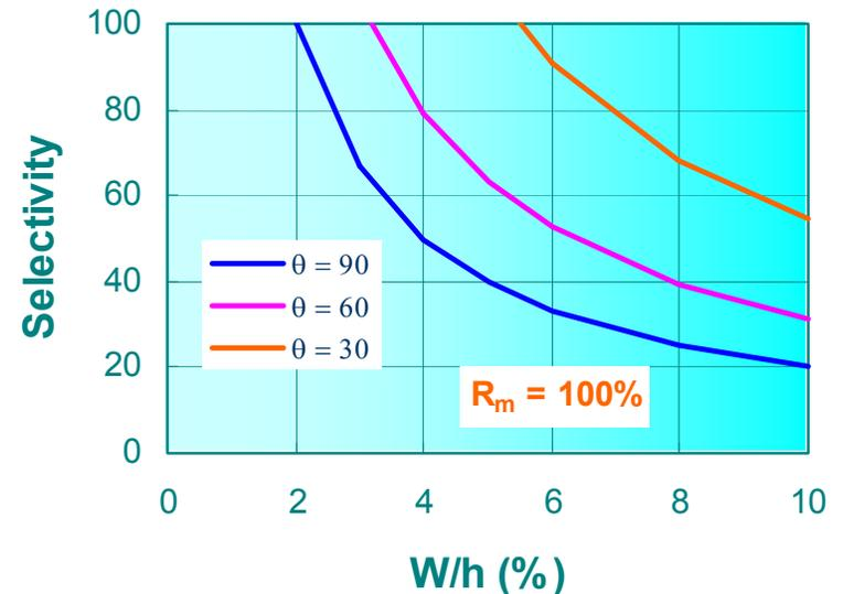
**Most mask material etches isotropically**
