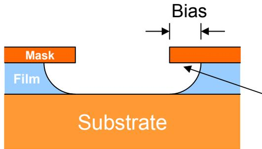
( $R_f = 1$ , pattern dimension is poorly defined)
