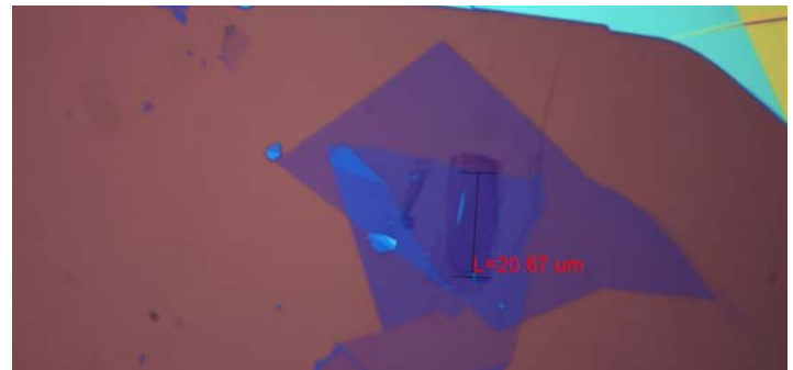
Top: Video of polymer stamp picking up a flake of boron nitride (outlined in red) Bottom: Two pieces of graphene sandwiched between boron nitride
